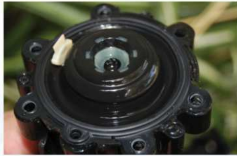
Remove debris from valve cavity
